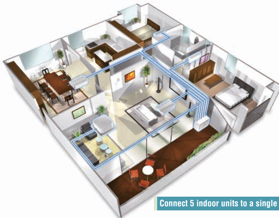
Up to 5 indoor units can be connected.
